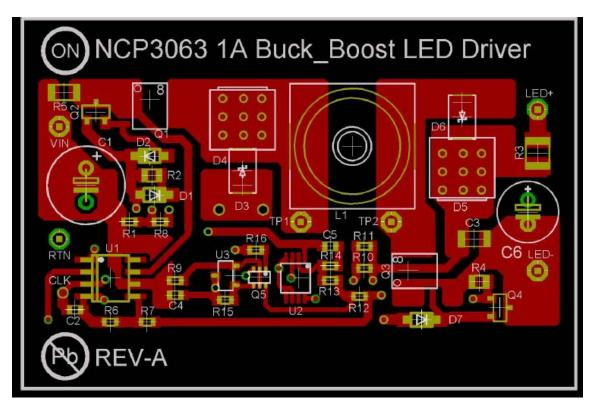
Figure 13. Top Side Component Layout
