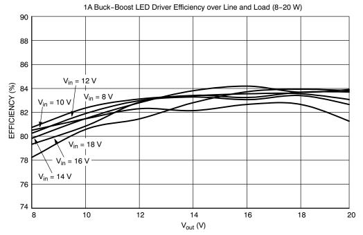
Figure 15. Efficiency Data Over Extended Input and Output Voltage Range
