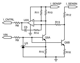
Figure 10. High Side Current Sensing Control Circuit
