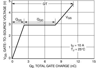
Figure 3. Gate charge characteristic of NTMS5P02
