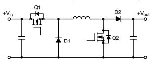
Figure 1. Buck Boost Converter
