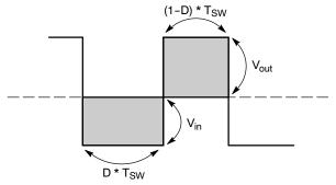
Figure 2. Voltage Waveform Across the Inductor
