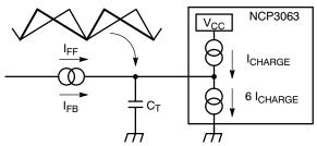
Figure 6. Current Injection into C<sub>T</sub> Pin Providing Continuous Duty Cycle Modulation
