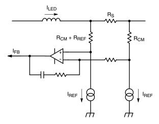
Figure 8. High Side Sensing Scheme
