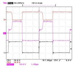
Figure 12. Boost Mode from 12 V<sub>in</sub> to 16 V<sub>out</sub>
