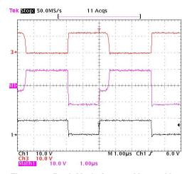
Figure 11. Buck Mode from 12 V<sub>in</sub> to 8 V<sub>out</sub>
