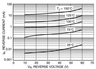
Figure 7. Reverse Leakage Characteristic of MBRD360
