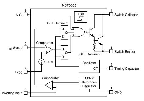
Figure 5. Block Diagram of NCP3063
